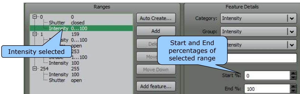
Any of the other "Channels" can be viewed and modified by clicking on them in the "Channels" pane. Click on "2: Colour Wheel". The "Ranges" pane now shows the DMX levels for the Colour Wheel channel.
