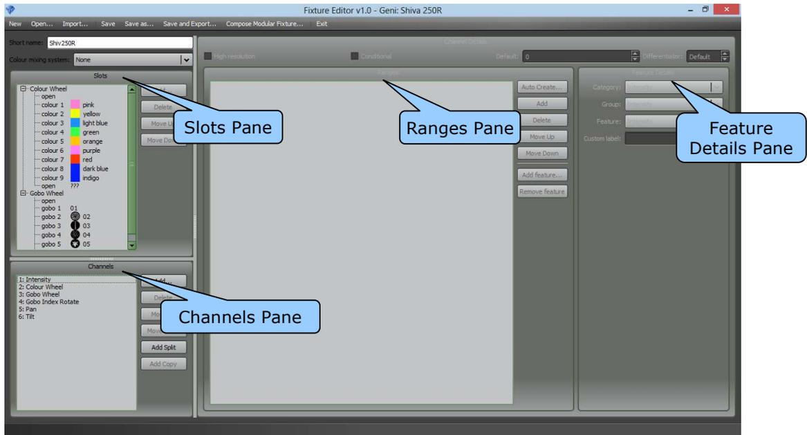
The "Channels" pane shows the 6 DMX channels used by this fixture.
