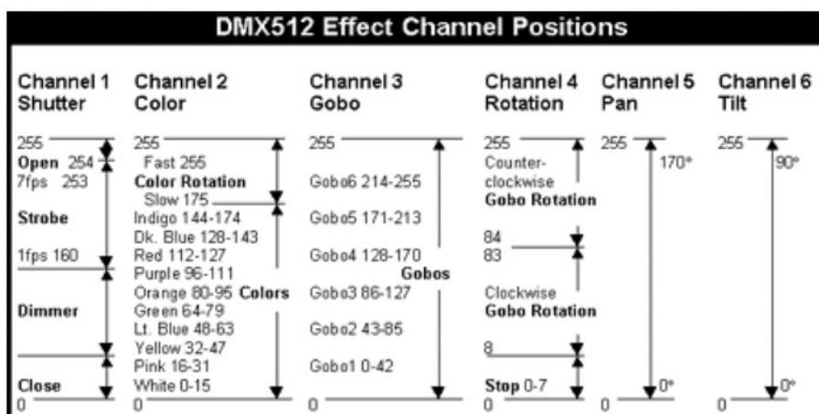
This fixture uses 6 DMX channels to control its functions. From the above chart we can see the DMX levels that determine the settings of each channel.
